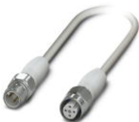
Sensor/Actuator cable, 4-position, PP-EPDM halogen-free, Gray RAL 7035, shielded, Plug straight M12, A-coded, on Socket straight M12, A-coded, Cable length: 0.3 m, Hygienic design, With high-grade steel knurl
