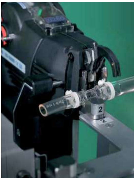
Exact positioning of cable ties.
