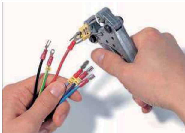
The sleeve applicator tool allows markers to be fitted after crimping.
