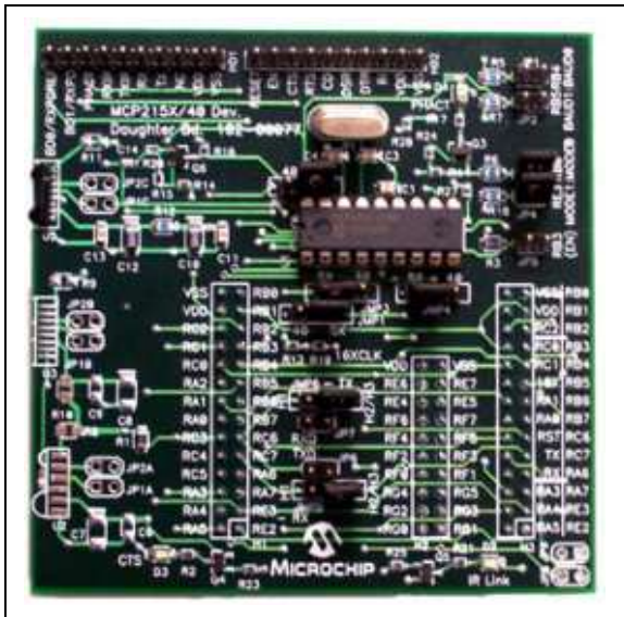
FIGURE 3-2: MCP215X/40 DEVELOPER'S DAUGHTER BOARD
