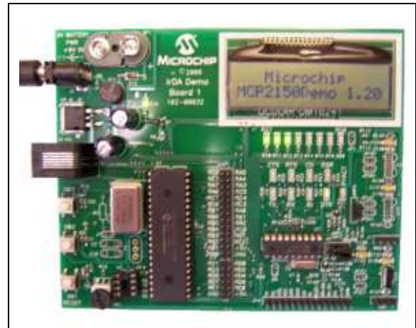
FIGURE 3-1: MCP215X/40 DATA LOGGER DEMO BOARD
