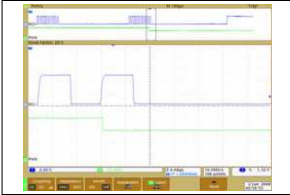
FIGURE 2-17: 5\text{ k}\Omega – Low-Voltage Decrement Wiper Settling Time ( V_{DD} = 2.7\text{V} ) ( 1\text{ }\mu\text{s}/\text{Div} ).
