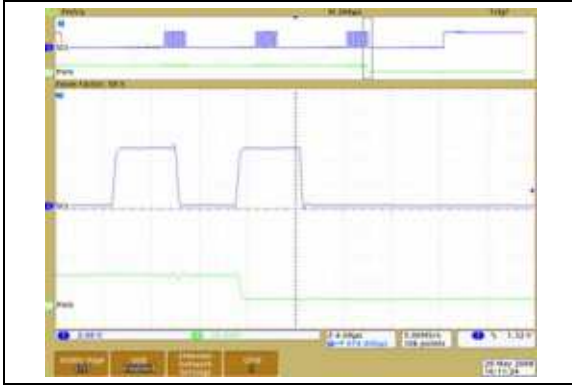
FIGURE 2-48: 50\text{ k}\Omega – Low-Voltage Decrement Wiper Settling Time ( V_{DD} = 2.7\text{V} ) ( 1\text{ }\mu\text{s/Div} ).
