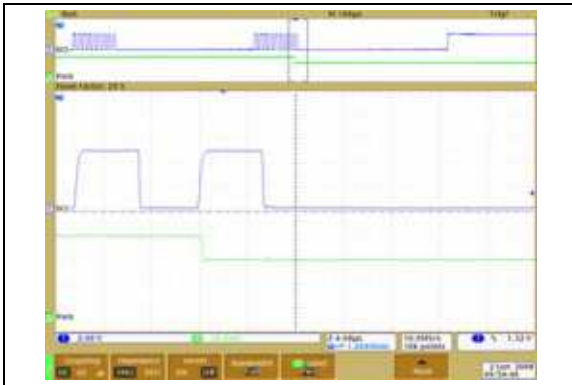
FIGURE 2-18: 5\text{ k}\Omega – Low-Voltage Decrement Wiper Settling Time ( V_{DD} = 5.5\text{V} ) ( 1\text{ }\mu\text{s}/\text{Div} ).
