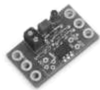
Field Installable Options 4-20mA / 0-10Vdc Signal Follower; Reversing Switch; Cover Kits
