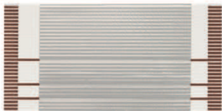
1mm tin plated, foil shielded FFC with conductors grounded to shield
