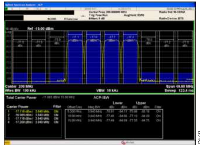
Figure 18. 4-Carrier WCDMA ACLR Performance, f_c = 200 MHz, f_{DAC} = 1228.8 MHz
