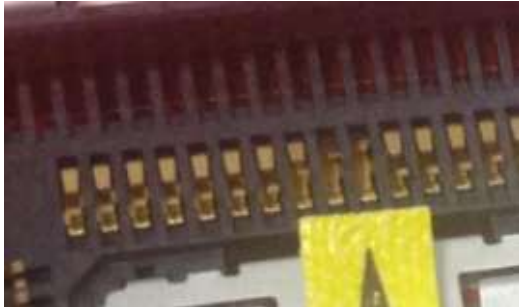
Figure 16. Example of Bent Contacts
