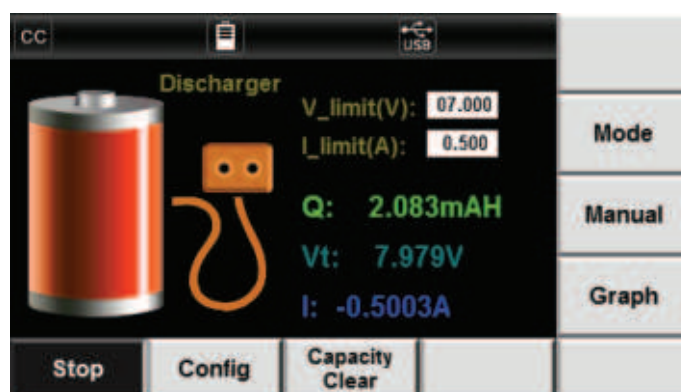
BCS6402 Discharge Set Up
