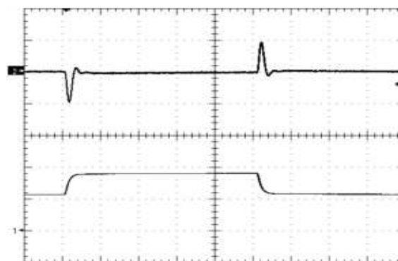
Figure 12. Load Transient Response (100mV/div), di/dt=0.1A/uS, 75% - 50% - 75% of full load, time scale: 200uS/div.
