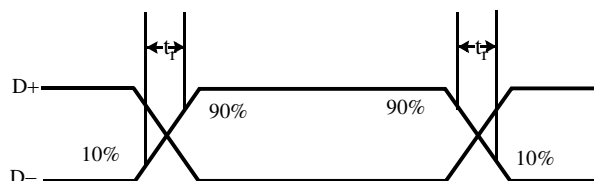
Figure 24-2. USB Data Signal Timing
