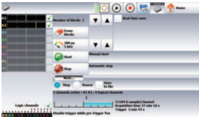
Comprehensive triggering capabilities: Configure triggers on analog and logic channels. Select from multiple combinations of thresholds, channels and conditions.
