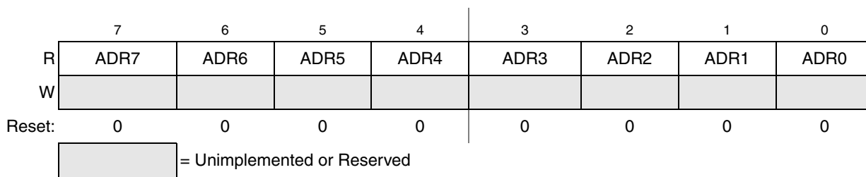
Figure 9-7. Data Result Low Register (ADCRL)
