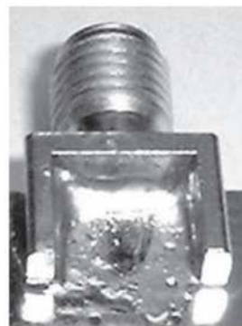
Figure 14. Soldering details of connector fingers to lower ground plane.
