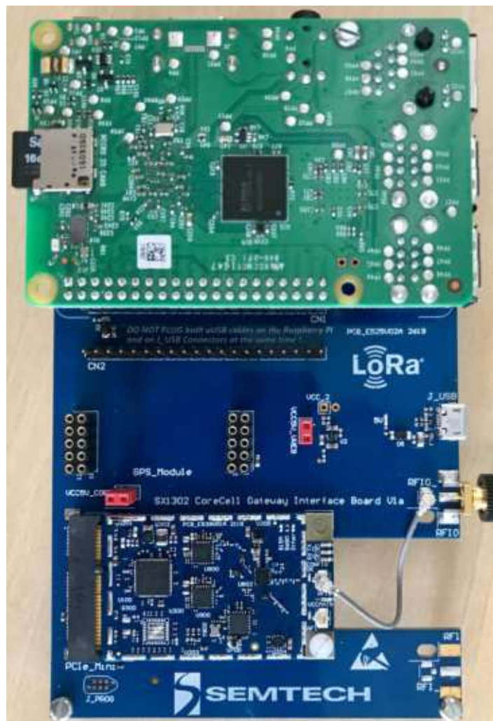
Figure 4: Raspberry Pi and Corecell GW Connection
