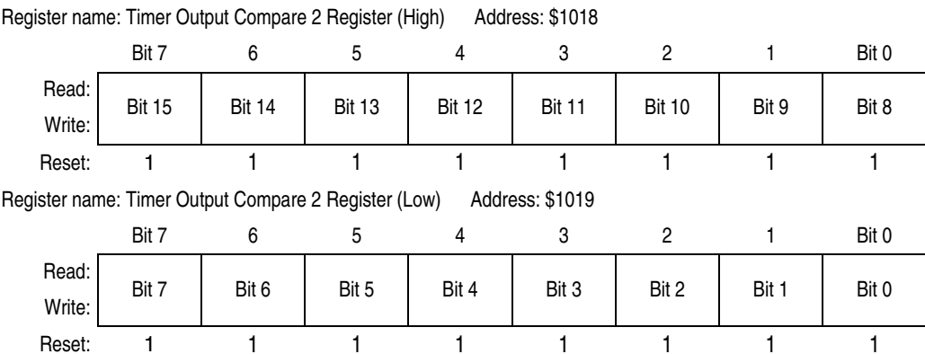
Figure 9-9. Timer Output Compare 2 Register Pair (TOC2)
