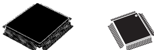
100 LQFP (14 mm x 14 mm) 64 LQFP (10 mm x 10 mm)
