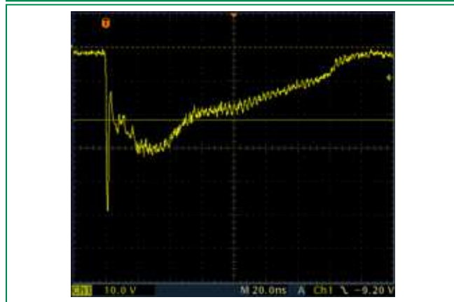
IEC 61000-4-2 -8 kV Contact ESD Clamping Voltage
