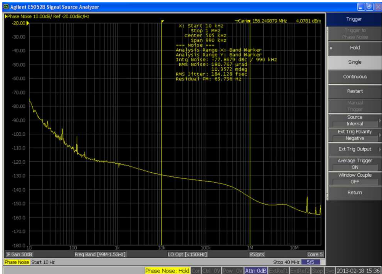
Figure 1. Si535/536 Typical Phase Noise at 156.25 MHz
