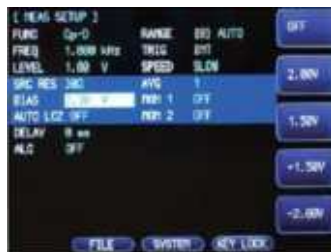
Internal Bias ( \pm 2.5V Adjustable) Ideal for Capacitive Components' Characteristic Tests
