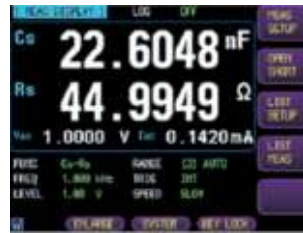
MEAS Display Parameter Setting and Four Measurement Parameters
