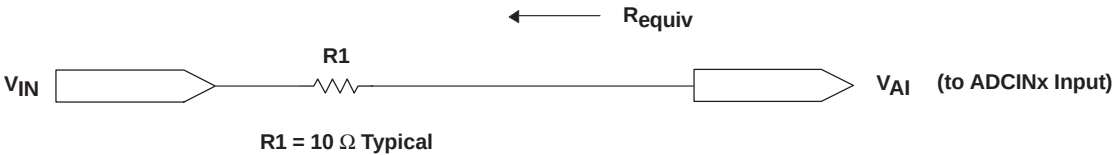
Figure 41. Typical ADC Input Pin Circuit
