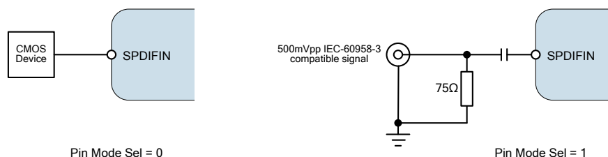
Figure 14 SPDIFIN Example External Connections
