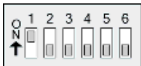
Figure B-08. RS-232 DIP Switch Settings
