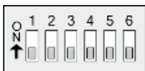
Figure B-13. RS-485 (2-wire) Half-Duplex DIP Switch Settings
