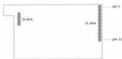
Figure 1-02. XStream OEM RF Module Pin Numbers (bottom view, pins protruding)
