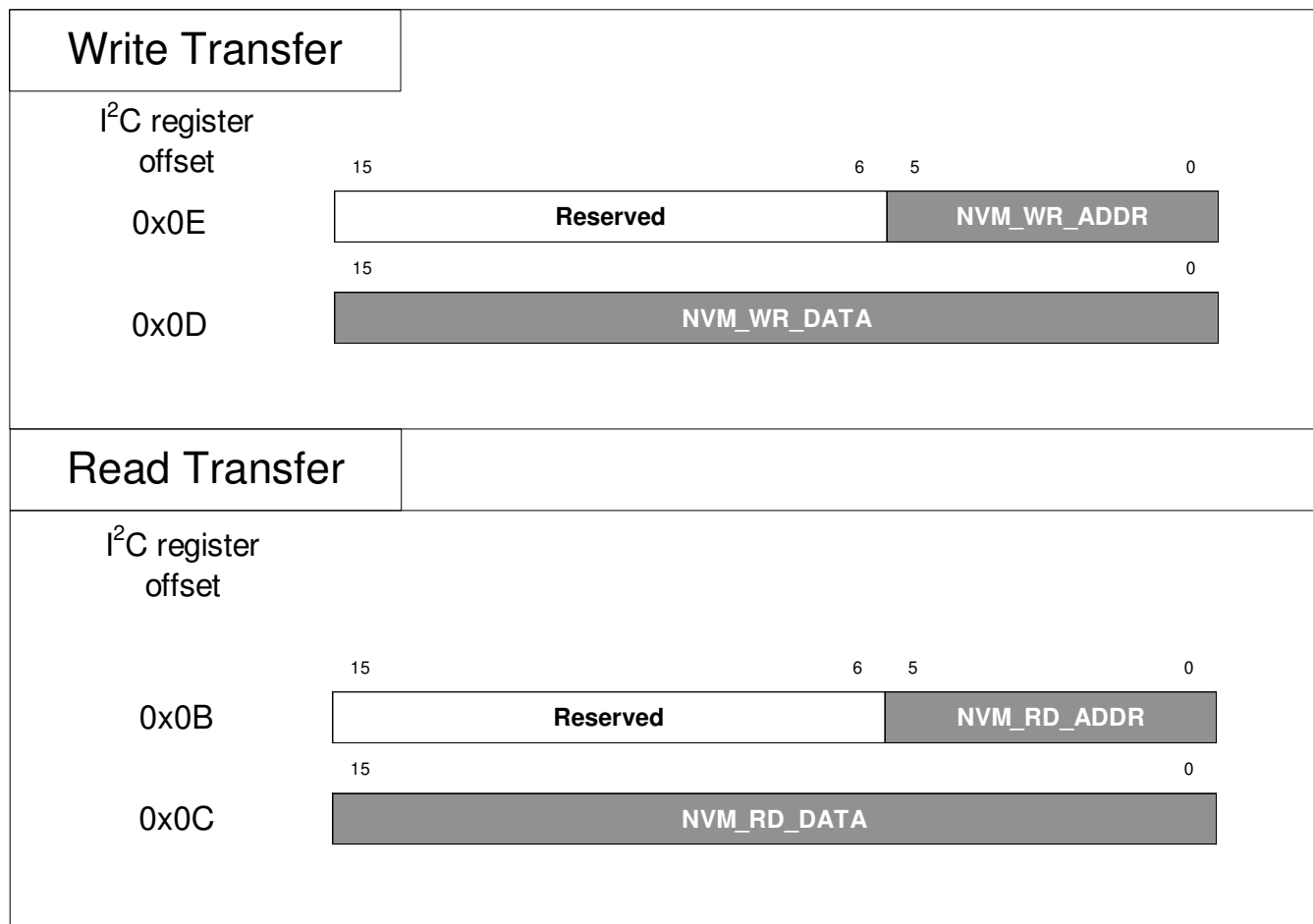
Figure 7-12. EEPROM Direct Access Using I 2 C
