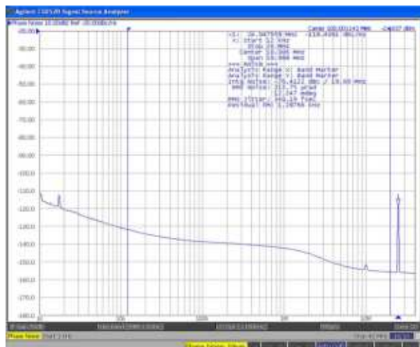
Reference: Crystal Closed-Loop Phase 100-MHz LP-HCSL Input 25 MHz Noise from 2.4-GHz VCO Figure 8-3. 100-MHz LP-HCSL Output for PCIe Application
