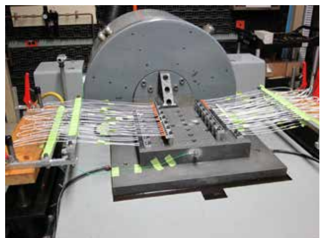
Figure 3 – Military Vibration Test - PIDG Terminals
