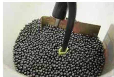
Figure 6 – Dielectric Strength Test – PLASTI-GRIP Terminal
