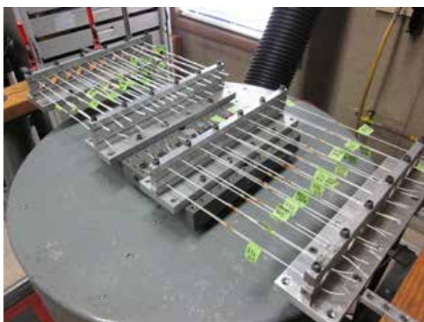
Figure 2 – Military Vibration Test - SOLISTRAND Splices
