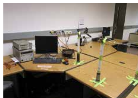
Figure 7 – Millivolt Drop Test – SOLISTRAND
