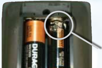
Corrosion you CAN see
