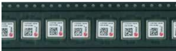
Figure 16: NINA-W101 module on tape orientation
