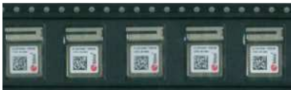
Figure 17: NINA-W102/NINA-W106 module on tape orientation
