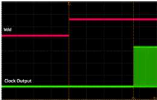
Figure 17. Startup Waveform vs. Vdd
