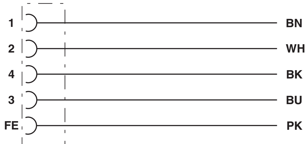
Contact assignment of the M12 socket
