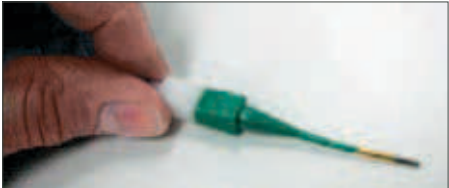
Plastic tool with contact in proper position.
