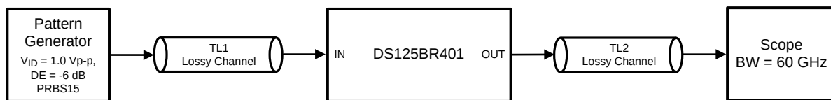
Figure 10. Test Setup Connections Diagram
