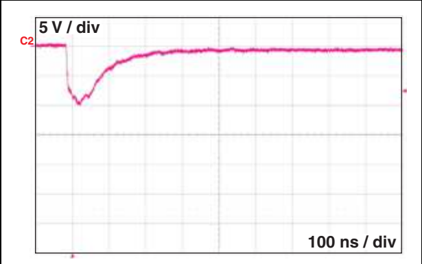
Figure 8. ESD response to IEC 61000-4-2 (-15 kV air discharge) ESDA12-1K
