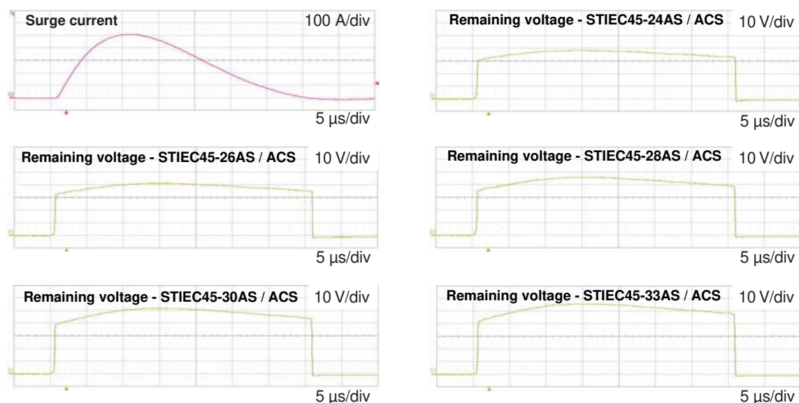
Figure 4: Clamping voltage at 500 A (1.2/50 \mu\text{s} - 8/20 \mu\text{s} )
