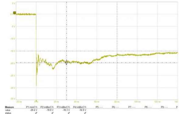
Figure 5. ESD response to IEC 61000-4-2 (-8 kV contact discharge)
