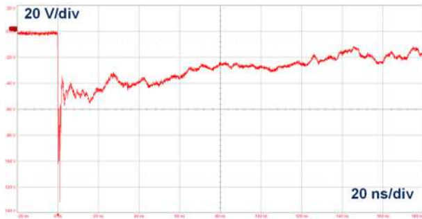
Figure 8. Response to ISO 10605 -C = 150 pF, R = 330 \Omega (-8 kV contact)
