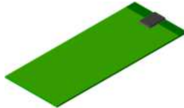
Cell phone config 1 ground plane (size: 40 x 100 mm 2 )
