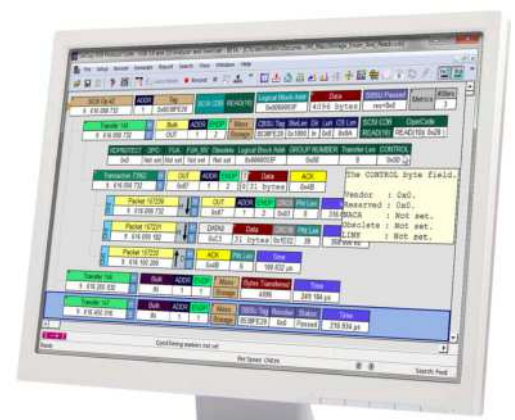
The CATC Trace display uses collapsible headers to group all packets that are part of a single transfer
