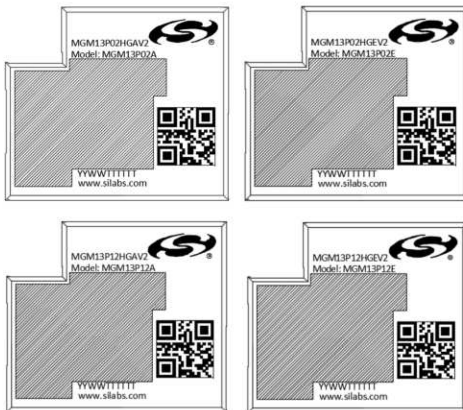
Figure 9.5. MGM13P Package Marking
