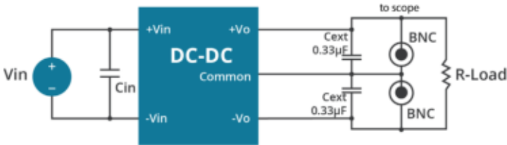
Figure 3 Measuring Output Ripple & Noise for Dual Output Models
