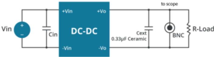
Figure 2 Measuring Output Ripple & Noise for Single Output Models
