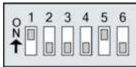
Figure B-11. RS-232 DIP Switch Settings
