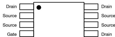
Figure 2. Pinouts for Single Die TSSOP
