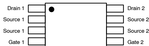
Figure 3. Pinouts for Dual-Die TSSOP
