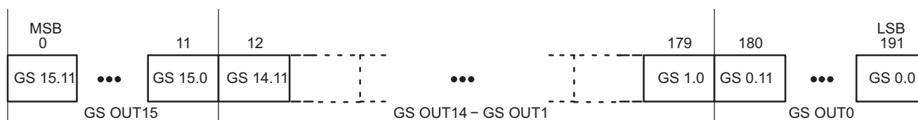
Figure 17. Grayscale Data Packet Format
