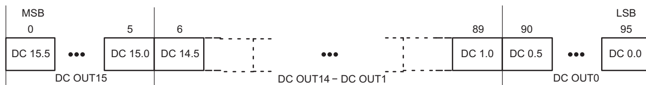
Figure 15. Dot Correction Data Packet Format
