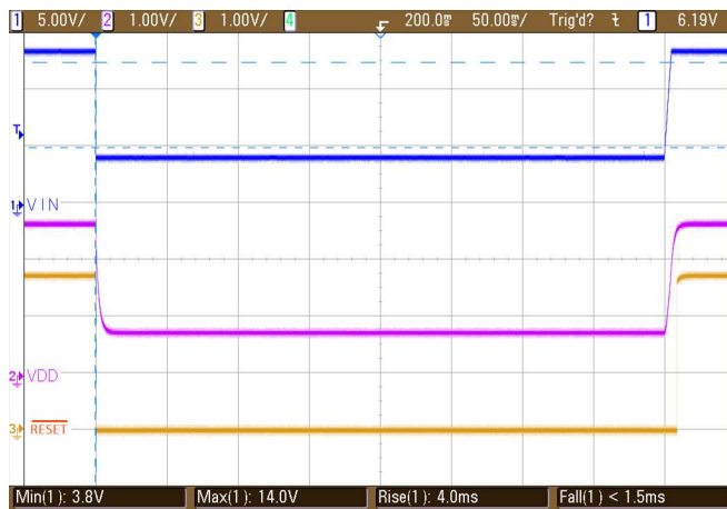
Figure 51. TPS3840-Q1 Warm-Start Test Pulse
