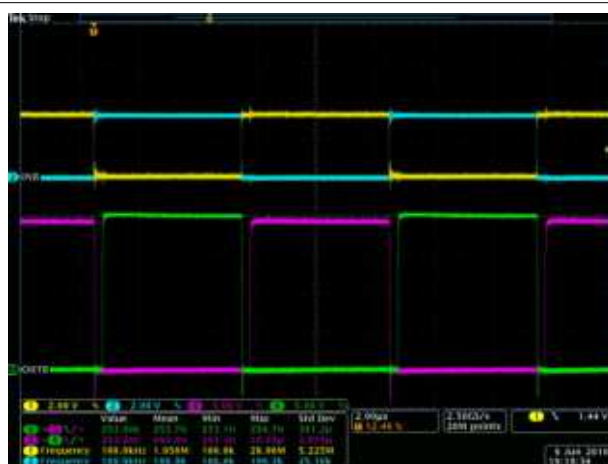
Figure 9-5. Bench Test Waveform for INA/B and OUTA/B
